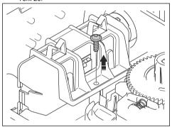
Push to detach the clips and lift up the battery holder.
