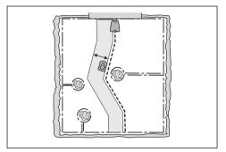
The corridor width is adjusted automatically. If it is necessary to adjust the corridor width manually for the product to operate satisfactorily, you can set the corridor width between 0-9. If guide corridor width is set to 0, the product straddles the guide wire. The factory setting is 6 for the boundary wire and 9 for the guide wire.
