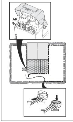
If the indicator lamp now is green, then the break is somewhere in the wire between the disconnected end to the point where the new wire is connected (thick black line below). In that case, move the connection for the new wire closer to the disconnected end (roughly at the middle of the suspected wire section) and check again if the indicator lamp is green.
