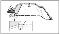
For slopes adjacent to a public road, put a barrier of minimum 15 cm / 6 in. along the outer edge of
