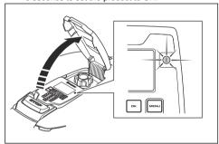
Push the ON/OFF button for 3 seconds to set the product to OFF. Make sure that the LED indicator goes out.
