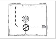
To make an island, isolate areas in the work area with the boundary wire. We recommend to isolate all stable objects in the work area.
